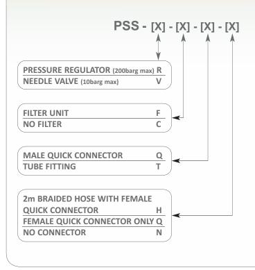
**NOTE:** PSS comprises the system chassis, two bulkhead connectors and piping for connection to the instrument, flow indicator and connecting piping to the instrument outlet bulkhead. An anti-static carrying case is included.
